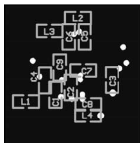
Figure 25. Bottom Layer Silkscreen
